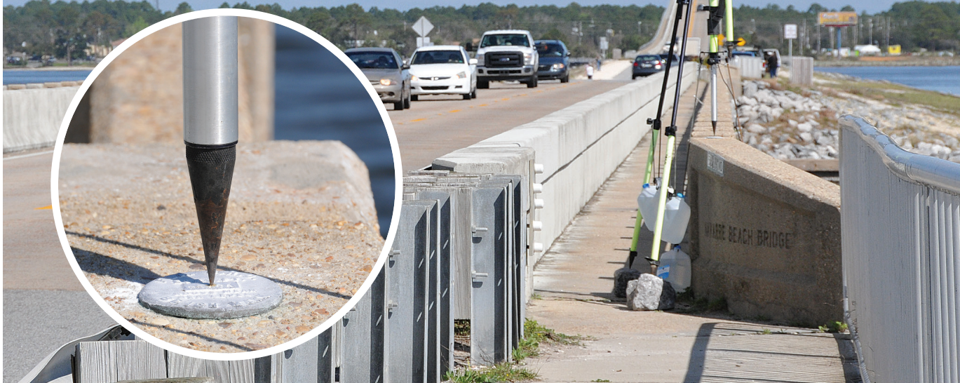
Navarre Beach Bridge was part of NOAA's National Geodetic Survey (NGS) on Saturday. Roy Anderson, Geotech surveyor for NOAA, was updating the bridge's global positioning coordinates disc which, through satellite access, can indicate any shift or movement of the bridge or the surface below the water. The NGS program provides the framework for all positioning activities in the nation. Its vision is for everyone to accurately know where they are and where other things are any time, any place.
